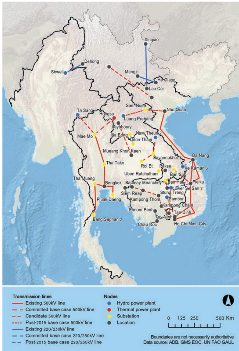
GMS Crossborder Power Transmission. Asian Development Bank. Greater Mekong Subregion Atlas of the Environment (2nd Edition) .
